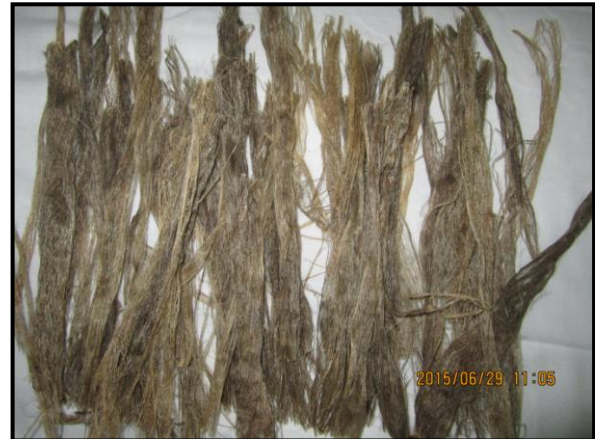
Fig: Udal fiber after treatment with NaOH solution
